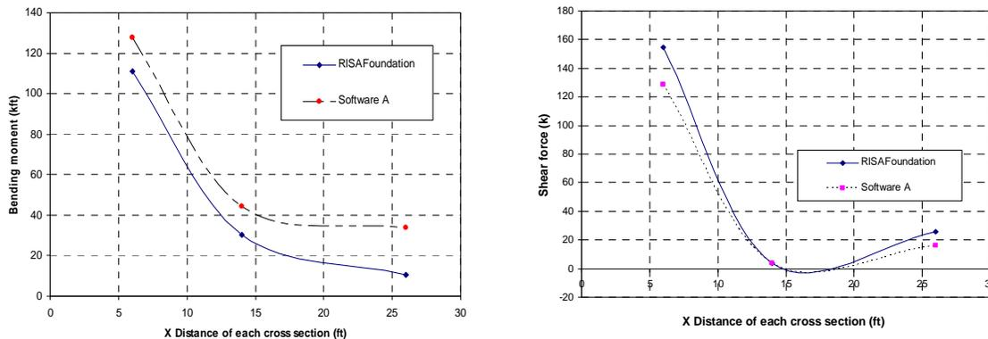
**Figure 5. A plot of moments/shears versus design cross sections obtained from various software**
