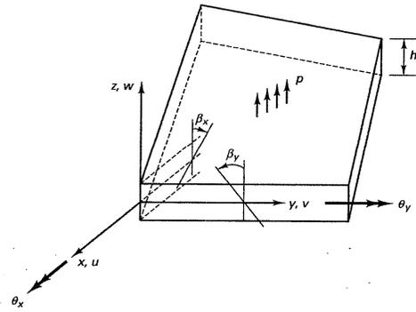
**Figure 2. Deformation assumptions in analysis of plate modeling including shear deformations**
