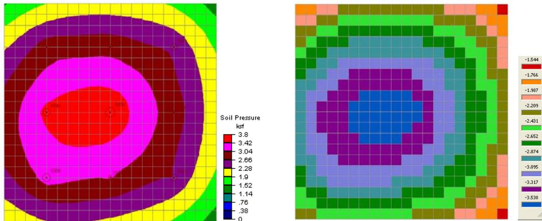
**Figure 4. Soil pressure plot (a) RISAFoundation (b) software B**
