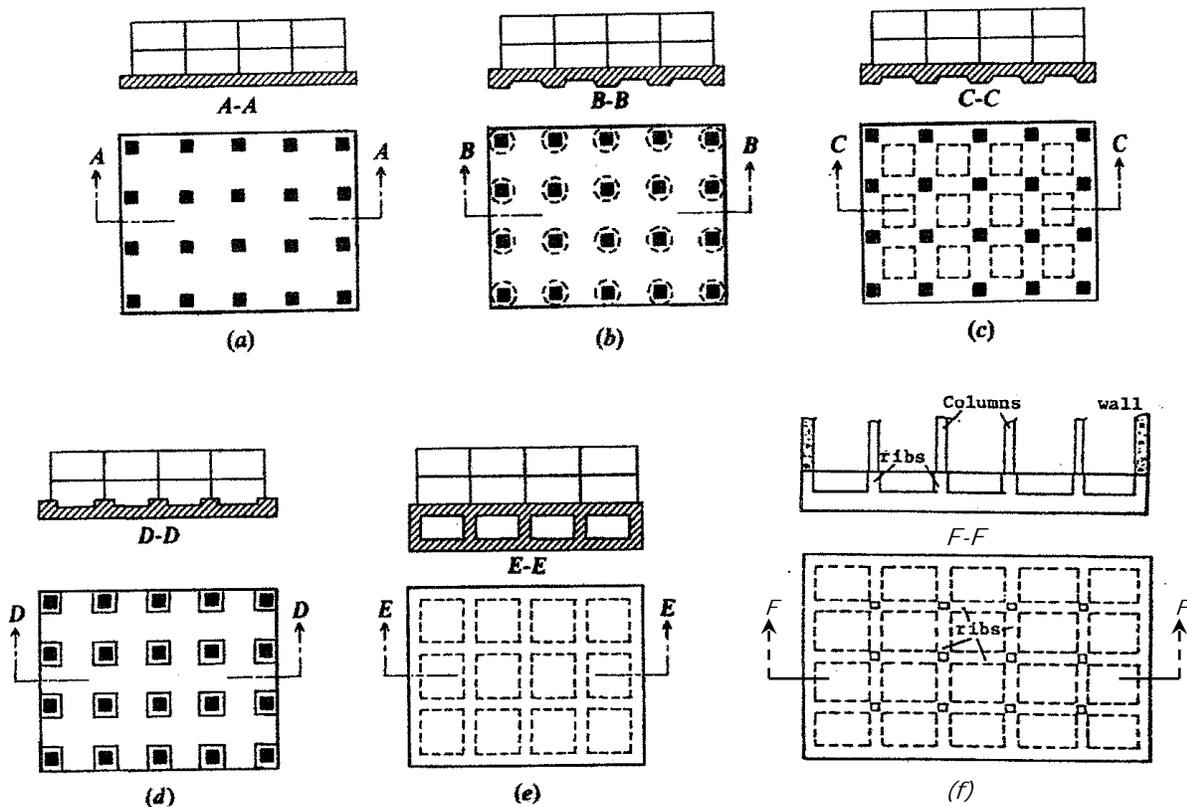
Figure 1. Common types of mat foundations (a) flat plate (b) plates with drop caps (c) waffle slab (d) plate with pedestals (e) cellular slab (f) rib slab
