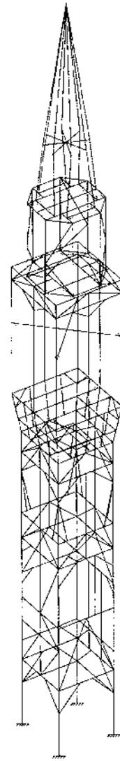
**Above, left:** New steel framing fits snugly within the existing 16' x 16' footprint.
