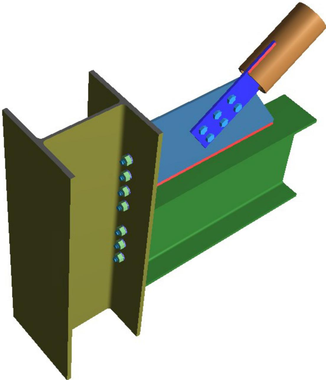
Lastly, the consideration of effective length of welds was also included in RISACONNECTION v4.0. Due to the uneven distribution of forces on welds on the face of tube columns as well as welds on brace End Tees, some lengths of weld must be ignored. In the interest of economy, the engineer should pay close attention to the proportion of HSS connections to ensure that as little weld as possible is “wasted”.
