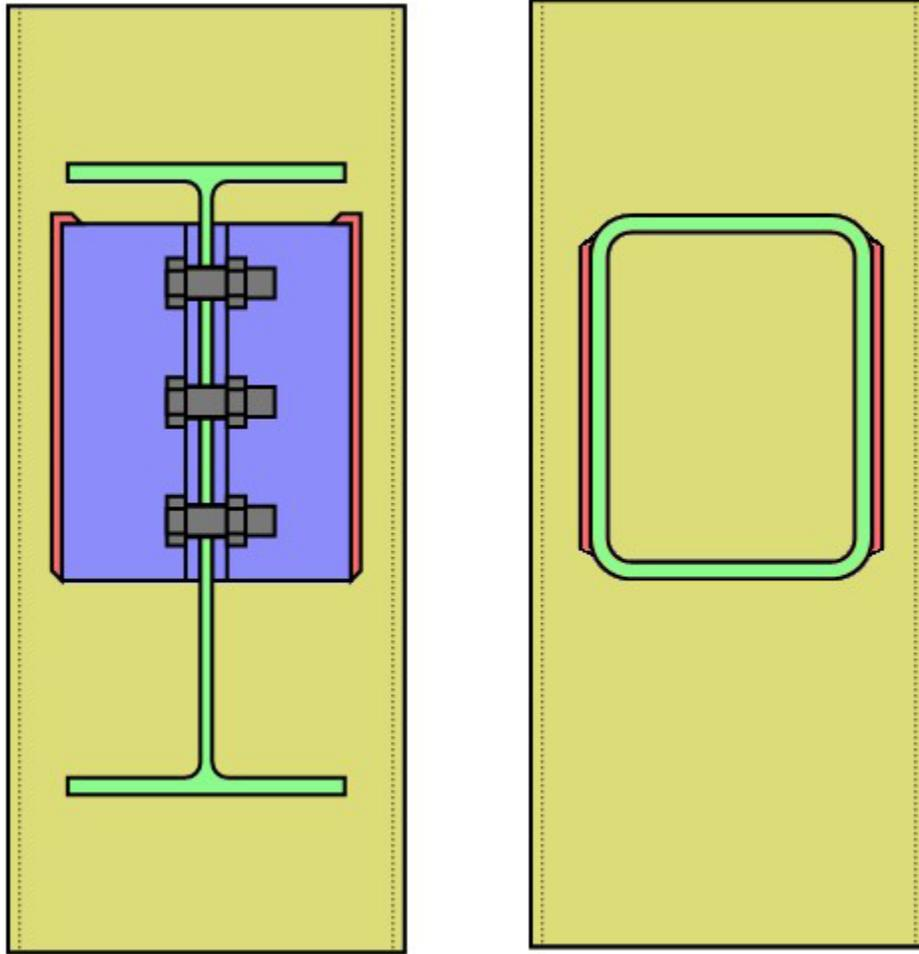
The moment due to eccentricity cannot be ignored either. When the chord/branch analogy is applied to this connection, the column can be checked for Wall Flexural Plastification and Sidewall Local Yielding where the moment capacities are compared against the net moment caused by both horizontal and vertical eccentricities on the connection.
