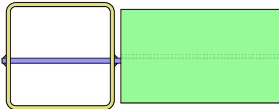
Section Cut (looking down) of Shear Tab Connection with Through Plate
