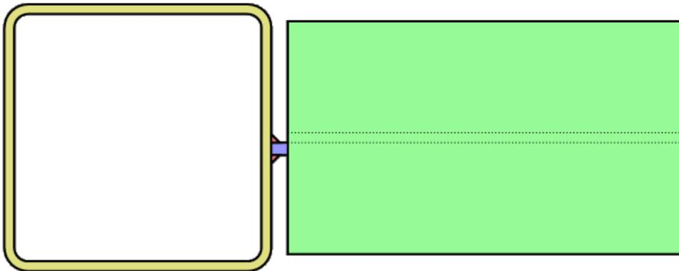
Section Cut (looking down) of Shear Tab Connection without Through Plate
