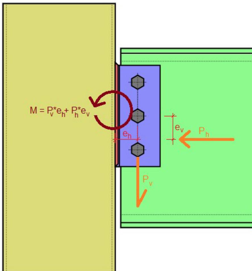
In this case, RISA draws a parallel between the way the clip angles attach to the face of the column and the way an HSS branch would attach to the face of an HSS chord in a truss. By using this comparison the column can be checked for Wall Plastification and Shear Yielding (punching) caused by the axial compression using the dimensions of the clip angles in place of the branch dimensions.
