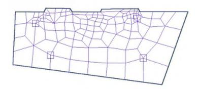
FIGURE A5-1 FLOOR PLAN SHOWING FINITE ELEMENT MESHING
