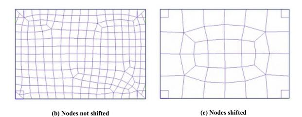
FIGURE A4.1-3 IMPACT OF NODE SHIFT ON MESHING
