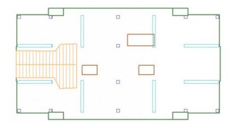
FIGURE 10.3-3 DESIGN SECTIONS FOR THE SLAB SUB-REGION
