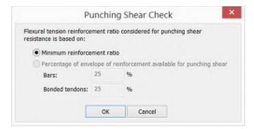
FIGURE 10.5-2 PUNCHING SHEAR CHECK REINFORCEMENT RATIO – AFTER REBAR DESIGN
