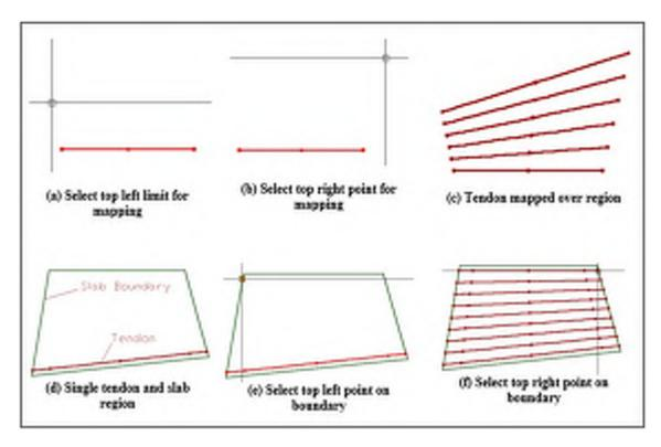
FIGURE 5.4-4 STEPS IN MAPPING A TENDON OVER A SINGLE REGION
