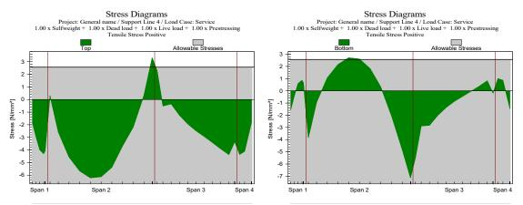
(a) Max tension 3.3 N/mm2, Allowable 2.6 N/mm2 - (b) Max tension 2.7 N/mm2, Allowable 2.6 N/mm2 Max compression -6.2 N/mm2, Allowable 11.9 N/mm2 - Max compression -7.1 N/mm2, Allowable 11.9 N/mm2
