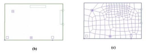
FIGURE B3.1-1 COMPONENTS WITH NODE PERMITTED AND LOCKED NODE SHIFT
