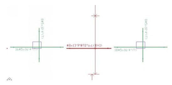
FIGURE 10.6-7 PARTIAL VIEW OF PLAN SHOWING DISPLAYED REBAR
