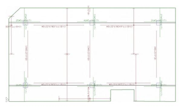
FIGURE 10.6-4 (1) SAMPLE REBAR DRAWING IN PLAN
