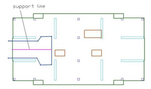
FIGURE 10.3-2 SUPPORT LINE FOR DIRECTION OF REINFORCEMENT
