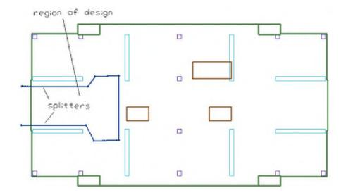
FIGURE 10.3-1 IDENTIFICATION OF A SLAB REGION FOR DESIGN
