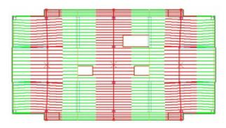
FIGURE 10.4-3 DESIGN SECTIONS ALONG Y-DIRECTION
