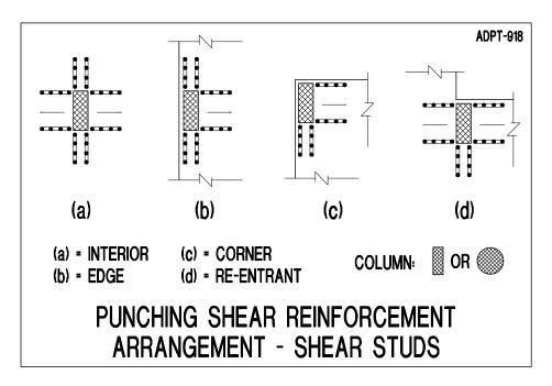
FIGURE 10.5-7 ARRANGEMNET OF PUNCHING SHEAR REINFORCEMENT USING SHEAR STUDS
