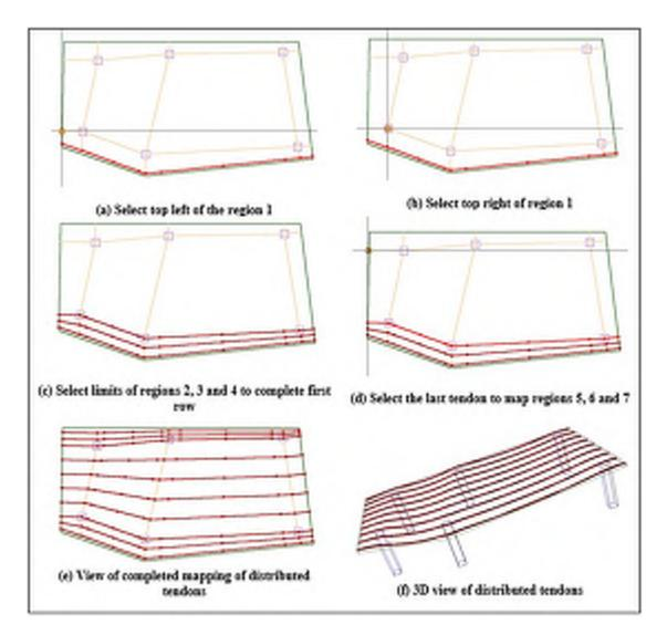
FIGURE 5.4-9 TENDON MAPPING OF COLUMN SUPPORTED SLAB
