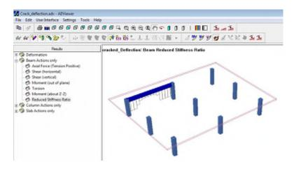
FIGURE 8.5-4 REDUCED STIFFNESS FOR BEAM
