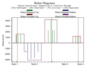
DESIGN STRIP REINFORCEMENT REQUIRED AND PROVIDED
