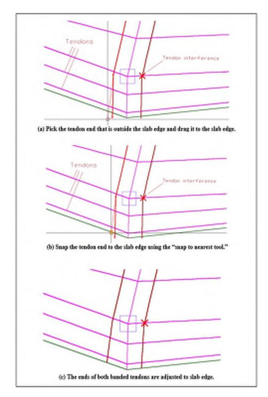
FIGURE 5.4-12 ADJUSTMENT OF TENDON END TO SLAB EDGE
