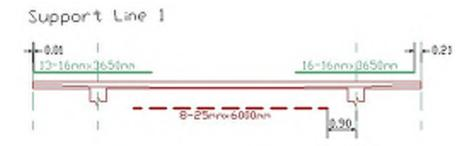
FIGURE 10.6-4(2) SAMPLE REBAR DRAWING IN ELEVATION
