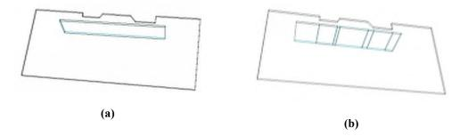
FIGURE B2.3-1 BREAKUP OF WALLS NEXT TO JAGGED SLAB EDGE
