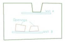
FIGURE B2.3-2 WALL "A" NEED NOT BE BROKEN UP, BUT WALL "B" MAY HAVE TO
