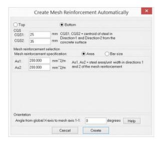
FIGURE 10.6-3 CREATE MESH REINFORCEMENT AUTOMATICALLY DIALOG WINDOW
