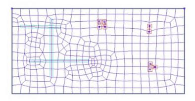
FIGURE B2-3 MESHING OF THE STRUCTURE USING NODE SHIFT
