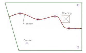
FIGURE 5.4-1 TENDON WITH CURVATURE ON PLAN
