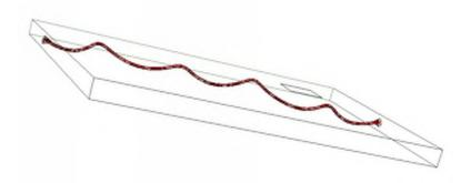
FIGURE 5.4-2 THREE-DIMENSIONAL VIEW OF TENDON WITH CURVATURE ON PLAN
