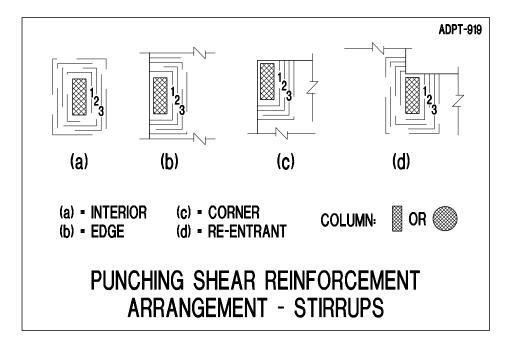
FIGURE 10.5-6 ARRANGEMNET OF PUNCHING SHEAR REINFORCEMENT USING STIRRUPS
