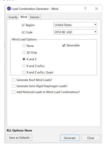
The LC Generator allows you to create load combinations quickly based on the code you select.
